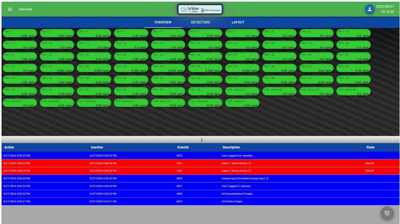
The screenshot shows the SkyView Overview page. At the top, there is a navigation bar with 'Overview', 'DETECTORS', and 'LAYOUT' tabs. Below the navigation bar is a grid of 67 detector points, each represented by a green pill-shaped button with a label (e.g., PS-7-1, PS-7-2, ..., GTD - Device 67) and a value of '0.00 ppm'. Below the grid is an event log table with the following columns: Active, Inactive, EventId, Description, and State.
