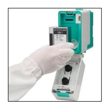
The PS-8 unit opens for quick and easy sensor replacement.
