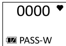
11. The SC-04 is now monitoring for gas in Measuring Mode. The Measuring Mode Screen displays the current gas reading.
