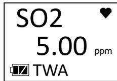
The TWA reading is the average reading *over the last 8 hours*. If 8 hours have not elapsed since the last time the TWA reading was cleared, the average is still calculated over 8 hours. The missing readings are assigned a value of 0. If **LUNCH** is set to **OFF** (factory setting), the TWA is cleared when the SC-04 is turned off.
