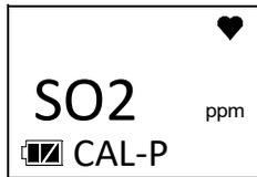
7. Press and release POWER MODE. The calibration value begins to flash.
