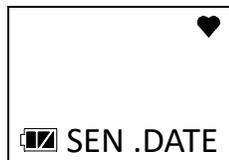
2. Press and release POWER MODE. The sensor replacement date displays.
