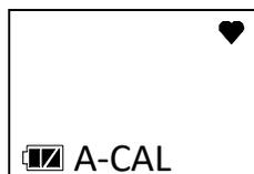
4. Press and release POWER MODE. The Auto Cal screen displays.
