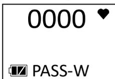
6. Use AIR to select each password number then press POWER MODE to save it and move on to the next number. To go back a number, press and hold AIR and POWER MODE for a few seconds.
