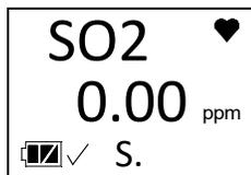
Heart Symbol: The heart symbol in the top right corner of the LCD indicates the operation status and flashes when normal. A microprocessor error causes the heart symbol to stop flashing or to disappear.
