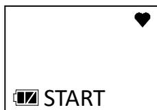
2. Press and release POWER MODE. The instrument begins its warm-up sequence.
