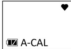
4. Press and release POWER MODE. The display shows the gas and its assigned calibration value (see pg.47 if the calibration value does not match the calibration gas cylinder's concentration).
