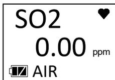
5. To return to the **AIR** menu without performing a fresh air adjustment, press and release **POWER MODE**.
