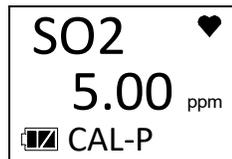
8. Use AIR to adjust the calibration gas value. The calibration gas value in the instrument must match the value listed on the calibration gas cylinder you are using. Limits on the calibration gas value are shown in the table below.
