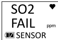
You cannot acknowledge the failure and continue to Measuring Mode. Replace the failed sensor as soon as possible.
