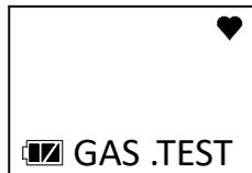
2. Press and release POWER MODE. The current gas reading displays. The bottom of the LCD alternates between “GAS.TEST” and “BUZZ.OFF”.
