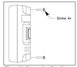
Figure 11: Unscrewing Case Screws
