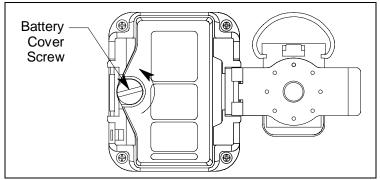
Figure 8: Unscrew Battery Cover Screw
