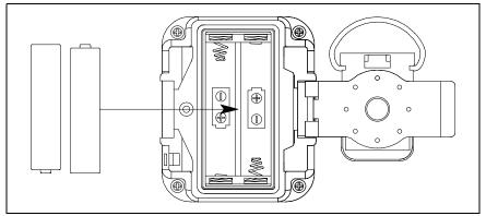
**Figure 10: Installing New Batteries**
