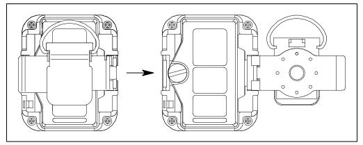
Figure 7: Releasing the Alligator or Belt Clip
