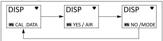
2. Press AIR to enter the **CAL.DATA** screen. The date of the last successful calibration displays.
