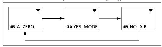
WARNING: Make sure that the instrument is in a known fresh air environment (an environment free of combustible or toxic gases and of normal oxygen content, 20.9%) before performing an auto zero operation. If you perform an auto zero operation in an area with gases present, the adjustment will not be accurate.
