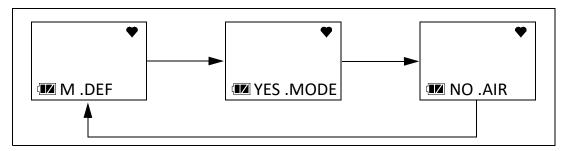
3. Press and release POWER MODE to perform a default operation. The instrument asks if you are sure you want to perform a default operation.
