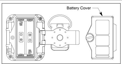
**Figure 9: Battery Cover Removal**
