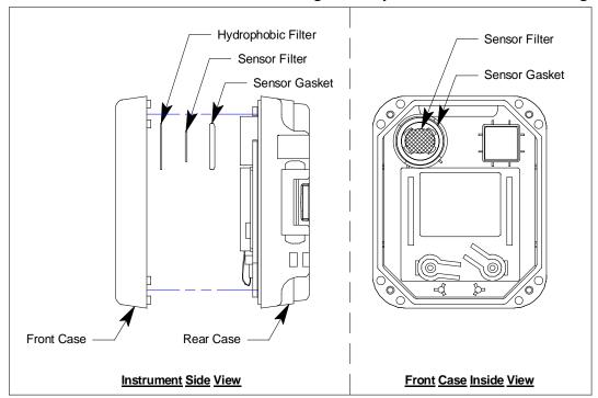
**Figure 13: Sensor Filter Location**
