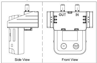
2. Use the tubing to connect the regulator to the inlet of the calibration cup (labeled "IN").
