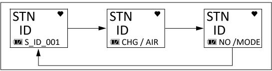
2. To change the Station ID, press and release AIR. The current Station ID flashes.
