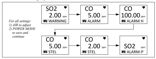
4. Use AIR to adjust the Warning setpoint. The alarm setpoint limitations are shown in the table below.
