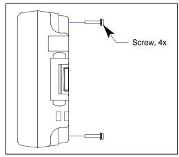
Figure 17: Unscrewing Case
