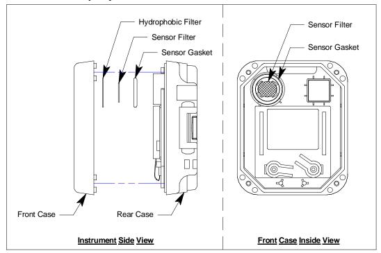
Figure 16: Hydrophobic Filter Location
