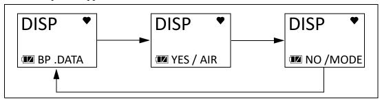
2. Press AIR to enter the **BP.DATA** screen. The date of the last successful bump test displays.
