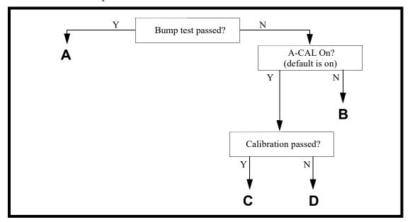
**Figure 6: Bump Test Flow Chart**
