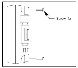
Figure 14: Unscrewing Case
