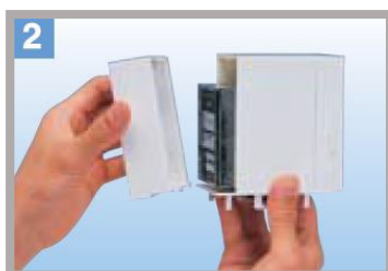
2 Remove back cover of the main unit.
