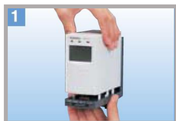
1 Remove the main unit from the base.
