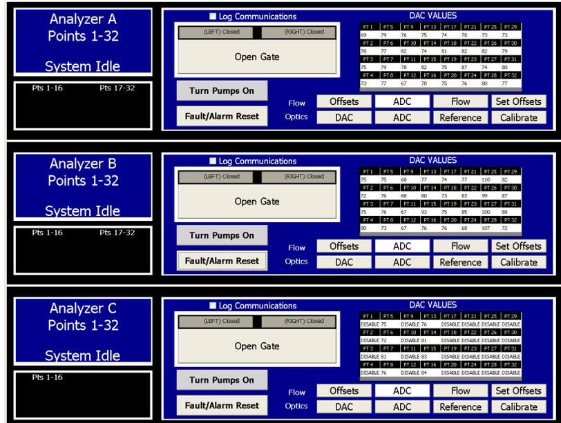
Select the DAC button for each analyzer and look for any “0” values or “255” values. Also, press the ADC button for each analyzer and look for any “0” values or “4095” values. If any point has these DAC or ADC values follow these steps first.
