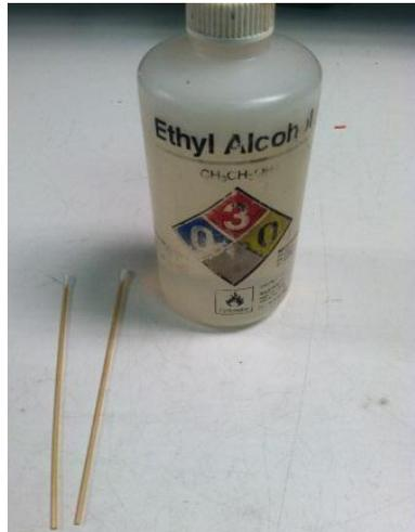
If the cotton end of the swab does not work the flat wooden end can also be used (see images below). Do not use anything metal or sharp to as this may damage or scratch the fiber or optic lens.
