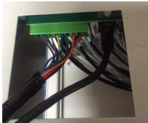
If the voltage at the green connector is below the required voltage, continue down to the pump panel and measure the voltage at the related analyzers fuse holder, red wire (+) and black terminal block (-)(see image below). Also verify none of the red lights are on, if one is on, this indicates a blown fuse and it must be replaced.
