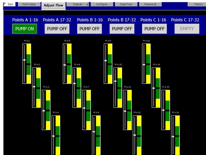
If the system is warning low flow on all points verify that the pump is on. This can be done by feeling the top of the pump to check if it is vibrating.
