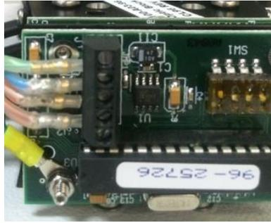
For the optic system to communicate properly the addresses on each block must be set correctly. A 32 point analyzer should be addressed 1 through 8 and a 16 point analyzer should be addressed 1 through 4. Using the optic block map on each analyzer and the chart below, with the optic covers removed, confirm the addresses are correct.
