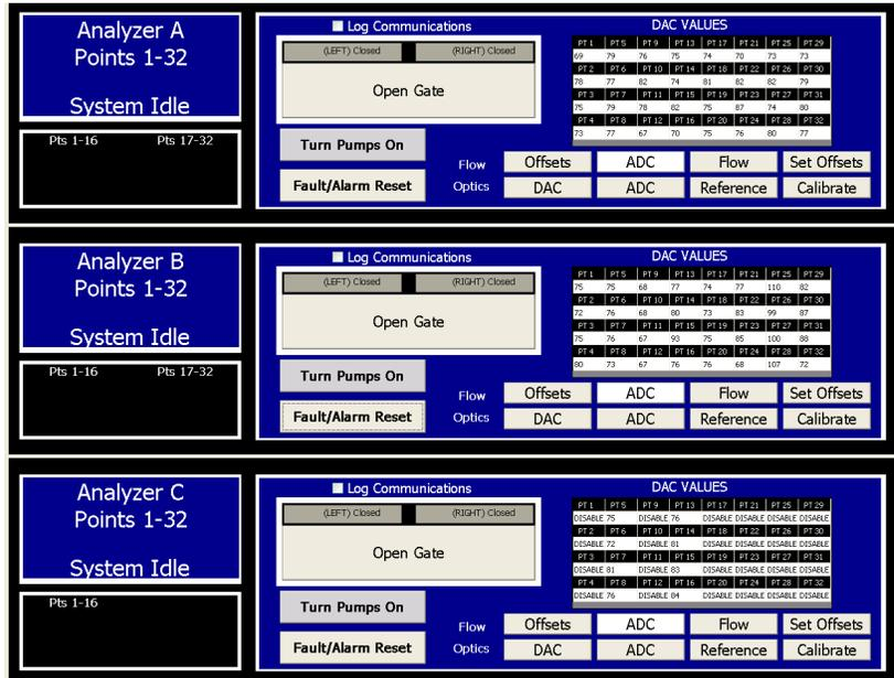
If a 0 value is found press the Set Offsets button for the related analyzer. If this does not resolve the issue check the flow system fuse light (See image below). If the red light is on, the fuse is blown and must be replaced.
