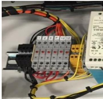
Next remove the rear panel and locate the flow system interconnect board (see image below). Verify that there is greater than 5.3V at the red (+) and black (-) wires. Also, verify that all interconnect board connections are secured.
