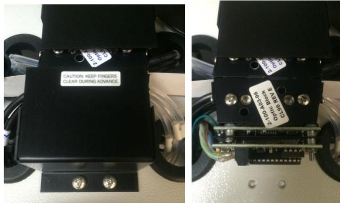
After the cover is removed, unscrew the two phillips screws holding the optic block down and pull the block over the optic alignment pins (see image below note; the pictures are showing a 16 point analyzer not a 32 point analyzer. In the case of a 32 point analyzer there will also be a black plate that lies between the lower 16 points and upper 16 points, the alignment pins and hold down screws will be longer.
