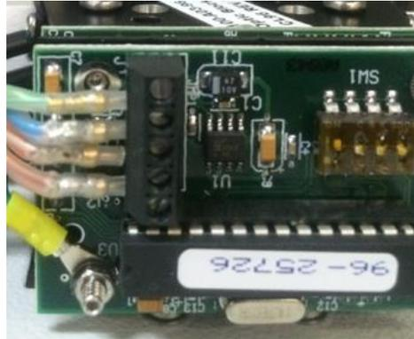
If the voltage is below 5.3VDC measure between the red (+) and the black (-) located on the green connector at the back of the analyzer (see image below). The voltage here should also be greater than 5.3 VDC.
