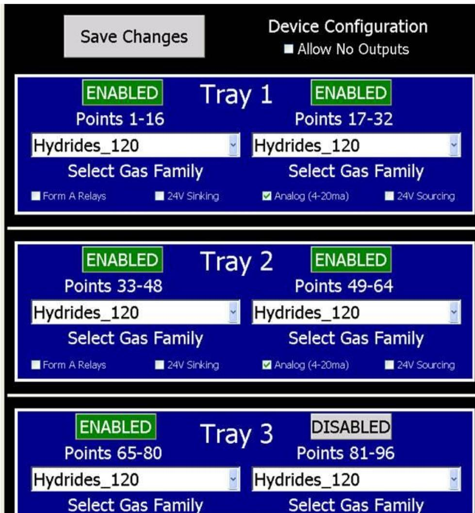
Verify that the correct boxes are checked for each active installed analyzer and check the allow no outputs box in the unit does not have any output modules. After any changes are made in this screen the unit should be power cycled. If this does not resolve the fault reset the communication between the PC and modules by unplugging the green cable in the control box (see image below) and plugging it back in.
