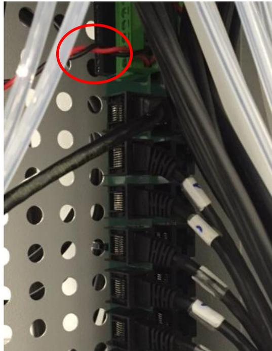
If all previous steps do not help locate a problem power cycle the transducer board that is producing 0 values by unplugging it and plugging it back in. Use the image below to locate the correct board. After the transducer board is plugged back in return to the system screen and press Set Offsets. If this does not eliminate 0 values please contact DOD Technologies technical support.
