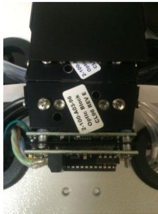
4. Remove the (2) screws holding down the optic block.
