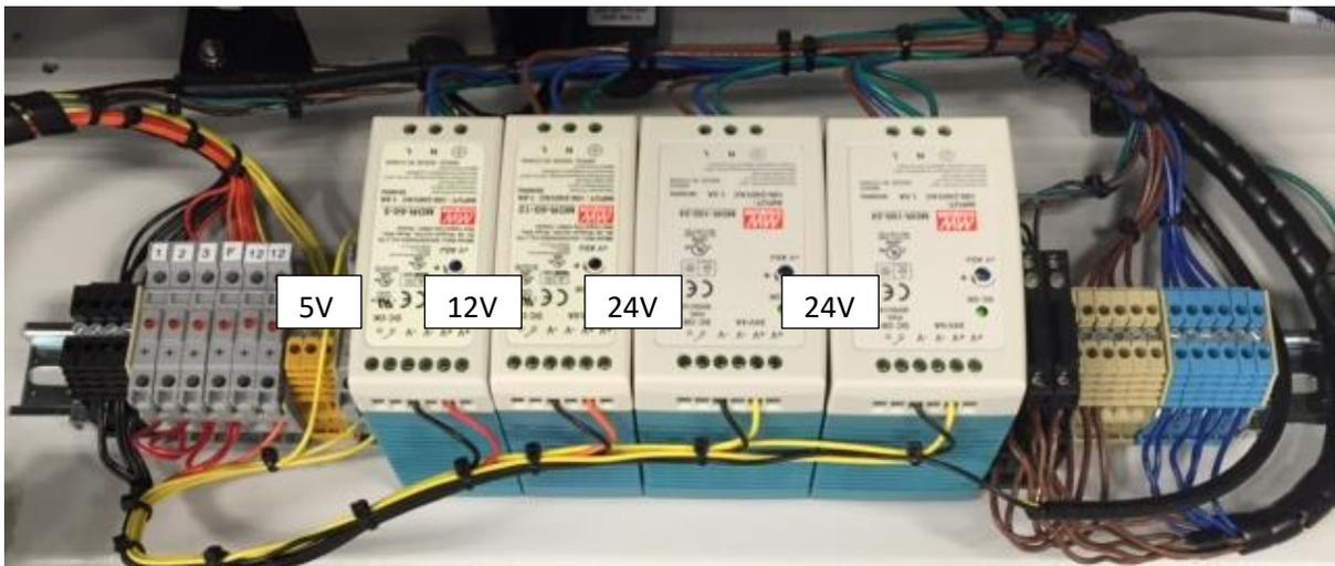
In the Control Box there is a row of terminal blocks mounted on the rear panel (see image below). The supply voltage for the PC and monitor can be measured at the yellow terminal block. The 12VDC supply can be measured at the orange terminal block and the 5VDC for the flow system can be measured at the red terminal block. The DC voltage verification should be done at the yellow terminal blocks mounted on
