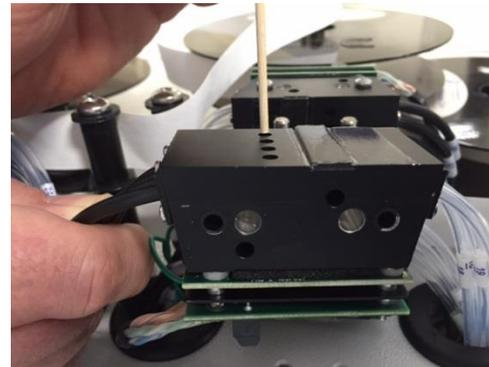
After the cleaning is complete re-install the optic block, Chemlogic cassette, and close the gate. Power cycle the analyzer by carefully disconnecting the green power connector on the back of the analyzer and re-connecting (see image below).
