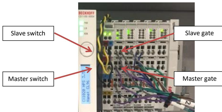
When standing in front of the analyzer the slave gate and micro switch are on the right and the master gate and micro switch are on the left (see image below).
