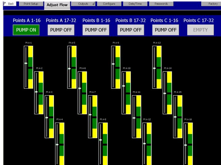
Next, verify that the flow system offsets are between 1000 and 1400 in the System screen and try to balance the flow again.
