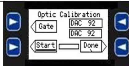
3. Keep pressing the tape against the block and covering Channel 2 opening. When the calibration is finished it will display a new DAC number
