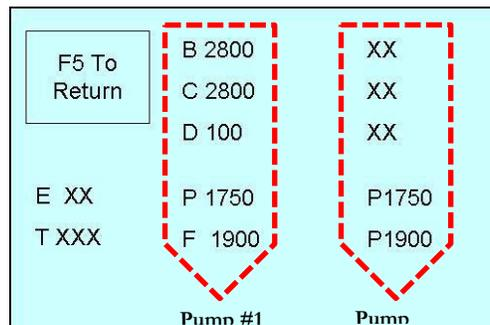
The diagnostic screen is formatted into 2 columns, the Left column is for when Sample pump 1 is operating and the right column is for when Sample pump 2 is operating.
