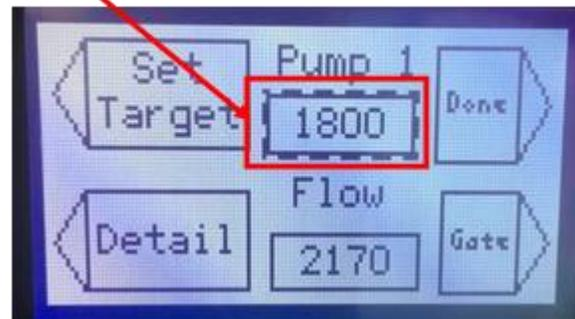
4. Using the numeric keypad, change the pump voltage value to 4000 then press enter.
