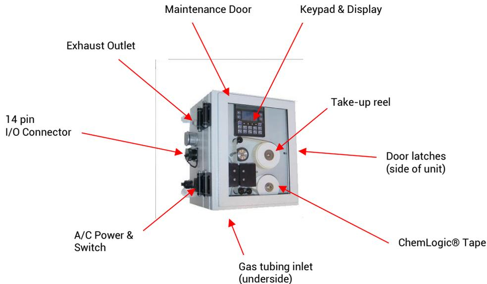
The system draws sample flow through the inlet on the bottom of the unit and across the ChemLogic tape then exhausted out on the left side of the CL1. Flow connections consist of “quick-connect” ports (2); one on the bottom (Inlet) and another on the left side for exhaust.
