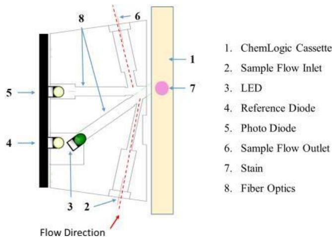
The optic system uses these 3 main components to monitor the ChemLogic cassette:
