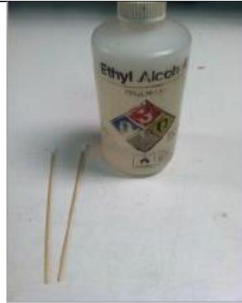
10. Dip the cotton swab into the alcohol and insert it in channel 2. It is very important to clean both lenses. Make sure to put the swab straight in to clean the first lens and angled downward to clean the second lens.
