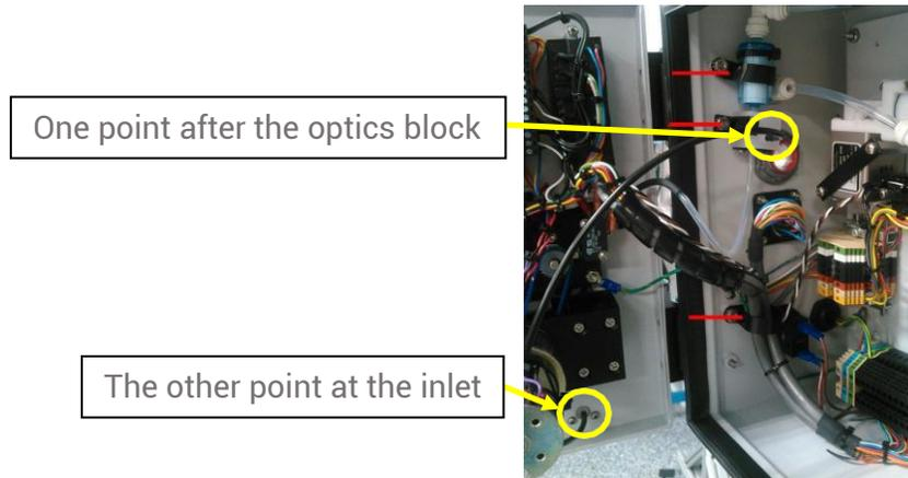
The difference in pressure that is monitored between these points is created by a small orifice at the inlet of the optic block. The pressure transducer reading (F) can be between 1600 and 2800 on a flow system that is performing correctly. If the (F) Value is < 1000 there is a leak in the system, or the pressure transducer has been damaged. If this value is above 3000 the optic block orifice is most likely clogged and needs to be cleaned. (see Appendix G for details)
