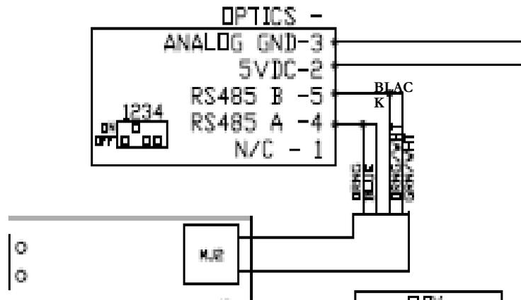
If wiring looks OK the try removing and reinserting the optic cable from the HMI (MJ2) and checking to see if this fault re-occurs. If this does not fix the fault, suggest replacing the HMI. (HMI's will come pre-programmed from the factory, but you must provide what gas files are needed for the CL1)
