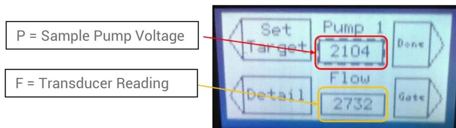
The Sample pump voltage (P) is represented on the HMI using a digital scale from 0 to 4000, 0Vdc = 0 and 12Vdc = 4000. If there are no problems with the Sample pumps or the shared flow path the P value should be between 1600 and 3200.
