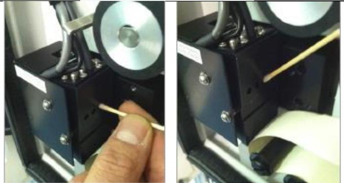
11. After the cleaning is complete re-insert the tape and put the back-plane block on. Press "Open/Close" and the gate will close.
