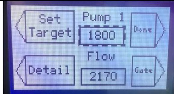
3. If the inlet flow is within 800 – 1100cc's then no adjustment is necessary.
