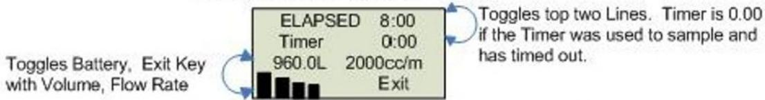
This display appears first when the pump has been stopped and turned off. The pump motor is off to enable the saved sampling data to be reported. Pressing the Exit key (down key) will return to the Main Display To allow resumption or setting of the pump.
