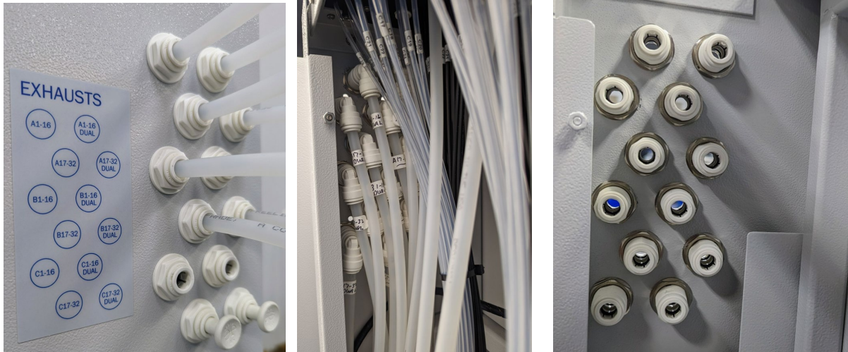
Images 1 2, and 3: Exterior and Interior Views from back of CL96 side panel. Tubing fittings/plugs and bulkhead fittings.
