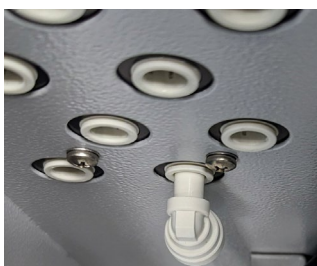
Image 14: Example of fitting not fully seated. Image 15: Example of fitting fully seated.
