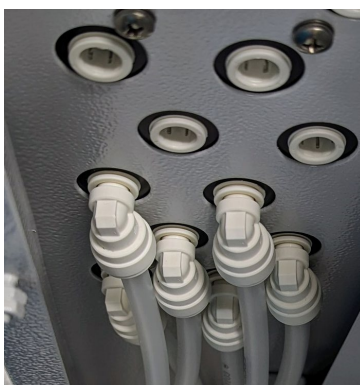
Images 16, 17, and 18: Interior Exhaust tubing/plugs (varies depending on options installed)
