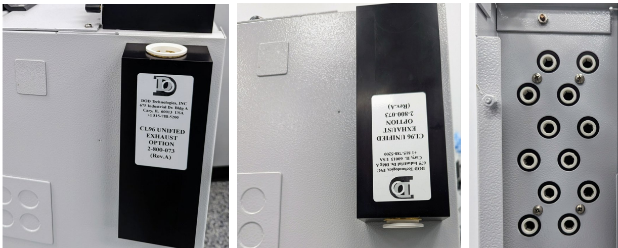
Images 10, 11, and 12: CL96 side panel view with (4) mounting holes the side panel.
